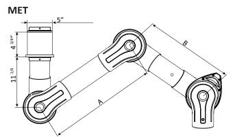
Add MTI bracket for ceiling mounting. Add MVK bracket for wall mounting.
