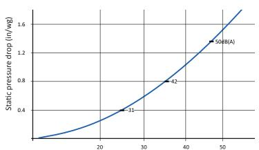
Static pressure drop is measured in accordance with ISO standard 5167-1. Air flow cfm Noise level is measured in accordance with ISO standard 3743. Indicated sound level refers to sound pressure level.
