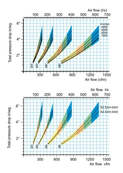
The black line shows the pressure drop for the arm when in the same position as in the design above. The area in the diagram shows the pressure drop at normal use. The field's tints show air velocity in the extractor according to below.
